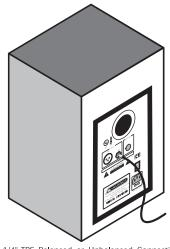
1/4" TRS Balanced or Unbalanced Connection
